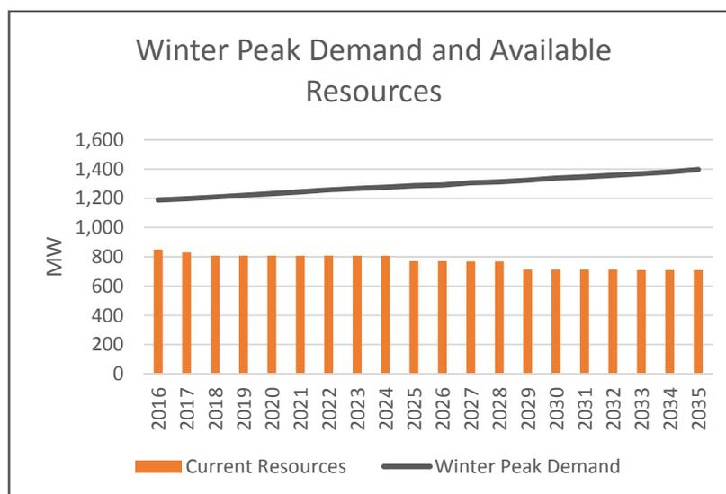
Retail loads at winter peak demand are forecast to grow from approximately 1,200 MW in 2016 to roughly 1,400 MW in 2035. The projected peak demand deficit for 2016 is 338 MW and forecast to grow to 688 MW, representing only half of peak demand needs, over the 20-year planning period unless additional capacity sources are secured. The peak load forecast includes reductions to peak demand associated with energy conservation measures from the 2009 Demand Side Management (“DSM”) assessment update.
