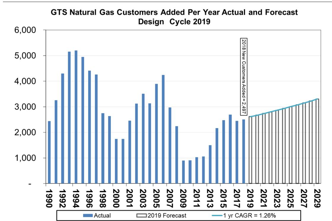
The weather-normalized load forecast does not indicate appreciable load growth in the short term. However, while annual loads have been (and are expected to be) relatively flat, growth in the number of customers on the system adds to the peak day requirement.
