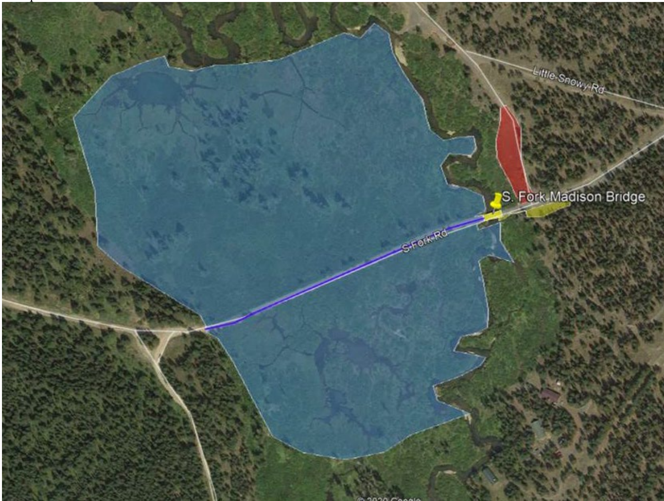
Figure 1. Proposed location of South Fork Madison River floodplain reactivation and habitat improvement project. The blue polygon shows the estimated causeway impact area, the red polygon shows the area of road with sedimentation impacts to be rebuilt, the yellow polygon shows the proposed improved parking area, and the dark blue line shows the length of the causeway across the floodplain of the South Fork Madison River.
