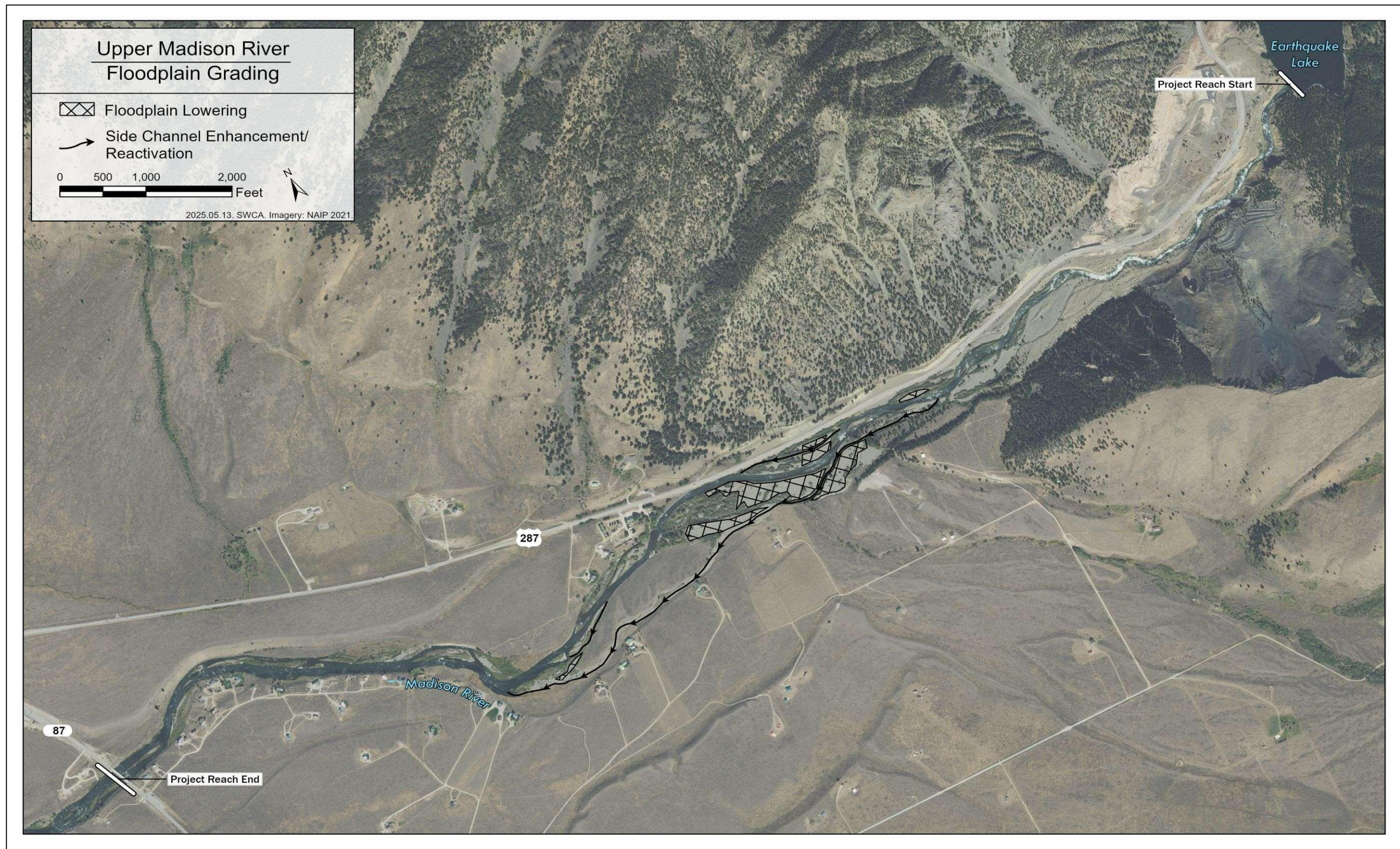
Figure 7. Floodplain grading alternative concept map with background imagery.
