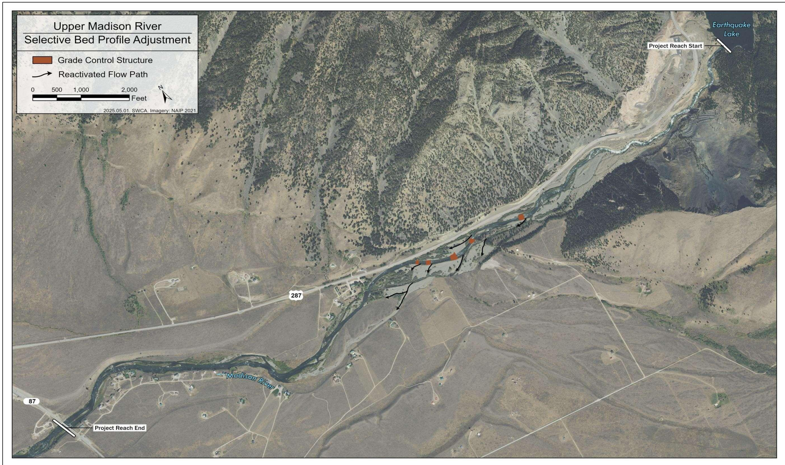
Figure 4. Selective bed profile adjustment alternative concept map with background imagery.
