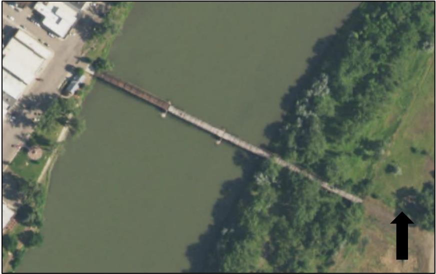
USDA aerial photo (2019) of old Fort Benton bridge with new decking on first span.
