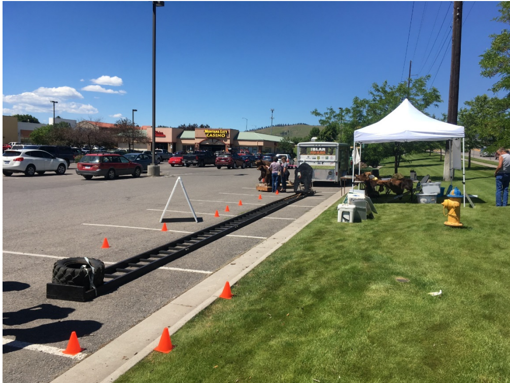
Bear attack simulator with winch tower and propulsion system early in the 2017 season
