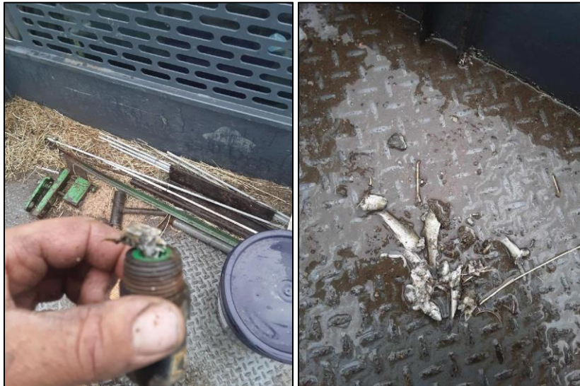
Photo 6. Evidence of plugged center pivot sprinkler heads, fed by the canal, as reported by Prickly Pear Simmental Ranch staff on September 27.
