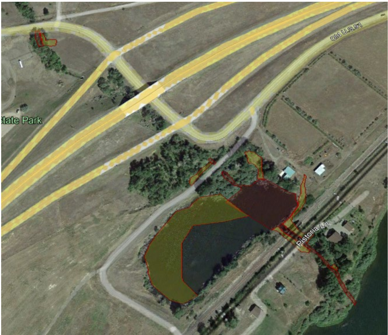
Figure 1. Map of Hardy Creek restoration project area. Red shaded areas = on-channel and floodplain disturbance areas. Yellow shaded areas = off-channel disturbance areas.
