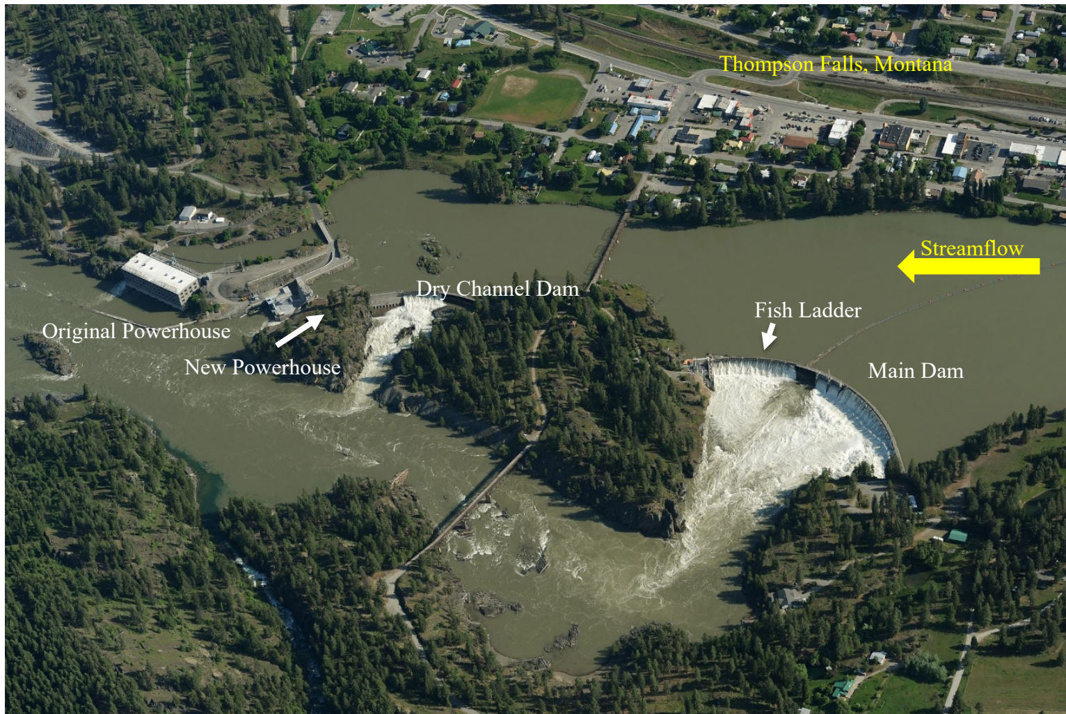
Photograph 1-1. Aerial photo of the Thompson Falls Project, taken June 2, 2014 with streamflows approximately 78,330 cfs (USGS Clark Fork River near Plains and Thompson River).
