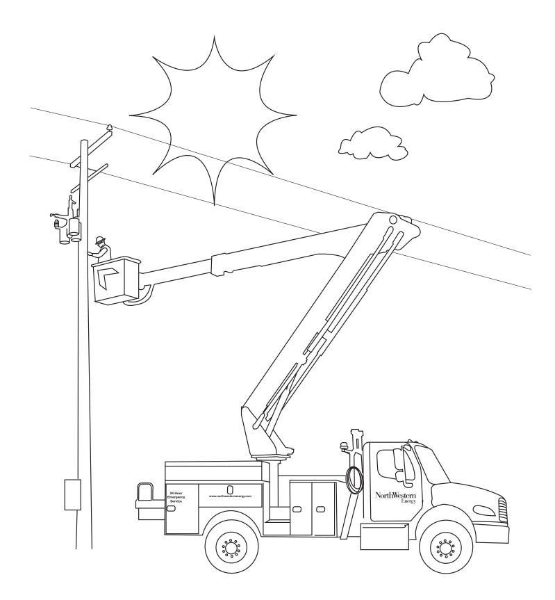
Line crews use bucket trucks with boom lifts to perform work. NorthWestern Energy has over 115 bucket trucks in South Dakota and Montana. Bucket trucks are a very important part of the fleet. Before bucket trucks linemen were climbing poles to install power and do repairs. Bucket trucks are designed to keep line workers safe and carry all of the tools necessary to do the job.
